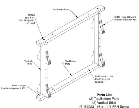
Mullion Kit. The C2312 Rollout Brackets and drawer slides should now be installed on the interior of the cabinet end panels and in corresponding locations on the Center Mullion Kit framework.
